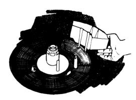
The self-cleaning filtering system and removable pump guard help eliminate prerinsing by removing food particles from the water.
